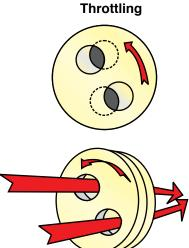
When the front disc is rotated, changing the alignment and relationship to the fixed back disc, the flow area and orifice size are affected, the result is either increase or decrease in flow.
