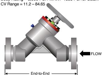
The MDIS Steam valve is designed for high pressure throttling of steam. The multiple orifice system is designed for long life in difficult applications. The standard valve has 1", 2", or 3" female NPT ends, with flanged or special ends readily available. Standard trim is Tungsten Carbide and designed for linear flow characteristics. Manual or electric actuation is standard.
