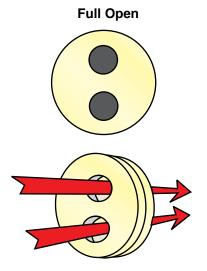
When the holes on both discs are aligned the valve is in the Full Open Position.
