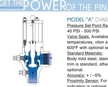
**OPEN** (STRAIGHT) The pin holds the piston in place until the set pressure is reached.
