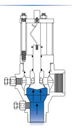
**CLOSED** (BUCKLED) When set pressure is reached, pin buckles to close valve.
